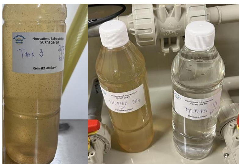
Figure 8. Left: Water from dirty BW tank. Right: Water from the inlet to the MF-pilot (MF Feed) and permeate water, sample after filtration (MF PERM).
