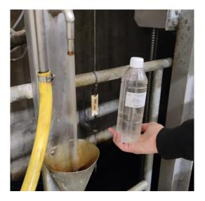
Figure 8. Sample bottle of 500 ml at sample collection site called PP100. Raw water coming out the tap for collecting raw water.
