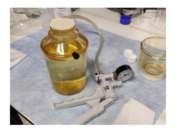
Figure 9. Suction filtration apparatus with handheld pump used to filter raw water samples to collect biomass on filter paper.
